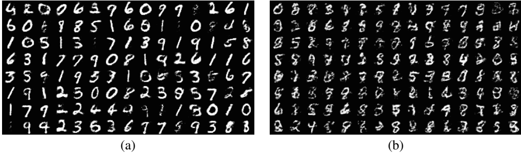
Figure 3: (a) Samples generated from a 5-layer deep DGA, composed of 3 shallow DGAs of 3 layers (1 hidden layer) each. The model was trained greedily by training the first shallow DGA on the raw data and training each subsequent shallow DGA on the output code of the previous DGA. (b) Sample generated from a 3-layer shallow DGA.
